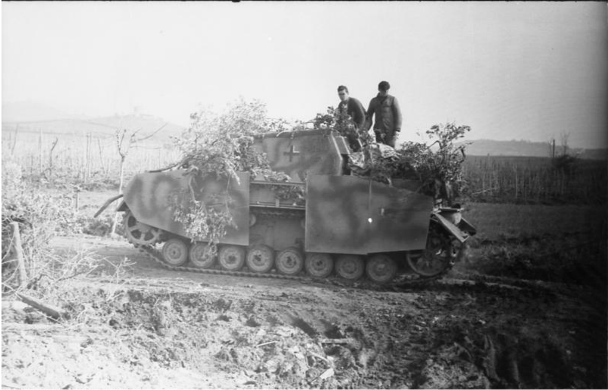
A few Sturmpfanz IVs were based on Ausf.F rebuilt chassis. Source: Wiki
