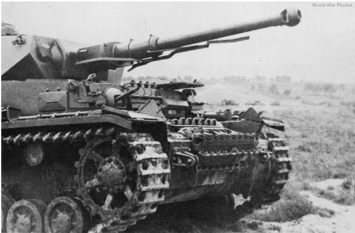
The Panzer IV Ausf.G, which was initially based on the Ausf.F. Source: www.worldwarphotos.info
