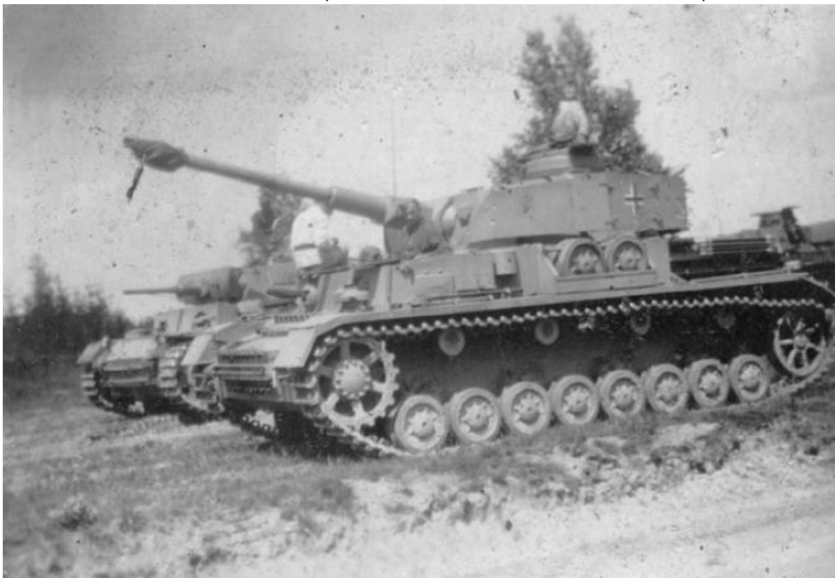
A Panzer IV Ausf.F armed with the longer 7.5 cm gun, possibly used as a training vehicle. Source: P. Thomas Panzers at War 1939-45
